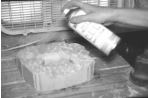
Mann Ease Release 200 is sprayed on mold.
